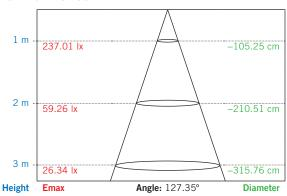
Note: The curves indicate the illuminated area and the average illumination when the luminaire is at a different distance.
